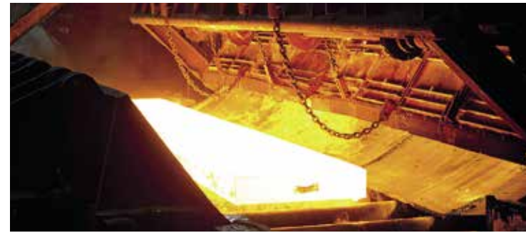
Slab discharged from reheating furnace heads back towards the roughing mill, NLMK Pennsylvania
